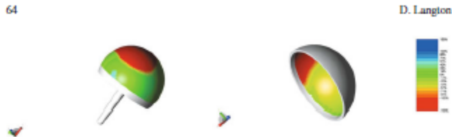
Fig. 5.1 Typical wear map of a failed hip resurfacing. Red areas indicate wear of greater than 10 \mu\text{m} . Volumetric wear rate was greater than 30 \text{ mm}^3/\text{year} in this case. Typically as is seen in cases of excessive bearing surface wear, blood Co concentration was 92 \mu\text{g/L} and Cr was 40 \mu\text{g/L} . Joint fluid levels showed the usual paradoxical concentration ratio associated with excessive bearing wear with Cr concentration of 11,000 \mu\text{g/L} and Co 4,500 \mu\text{g/L} . Gross metallosis and osteolysis was encountered at revision surgery though soft tissue necrosis was not extensive. Note that even with such elevated wear rates a large proportion of the bearing surface remains within the as-manufactured form ( green areas )
